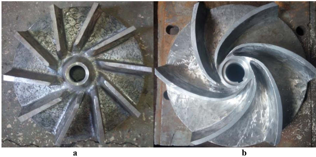
Fig. 3. Impeller of the TFP 125-50 torque-flow pump: a – base impeller; b – proposed impeller
