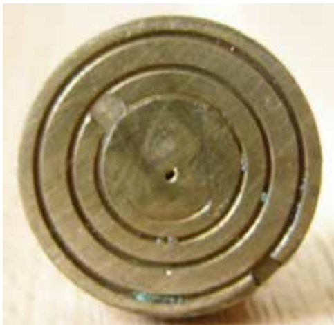
Common type of plunger heel wear
