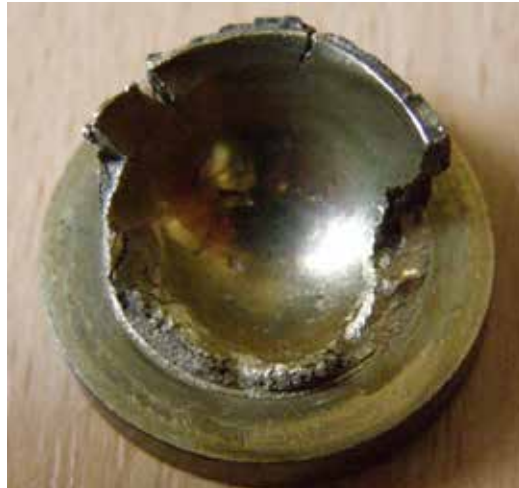
Fig. 5. Heel separation from the plunger bore
