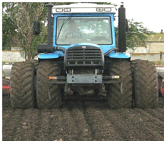
Fig. 5. Tractor KhTZ-17022 with dual tires 23.1R26D
