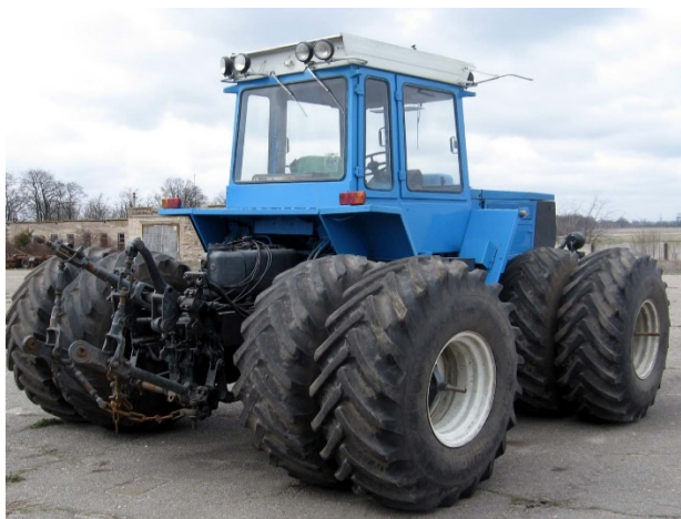
Fig. 4. Tractor KhTZ-16131 with dual tires 23.1R26D
