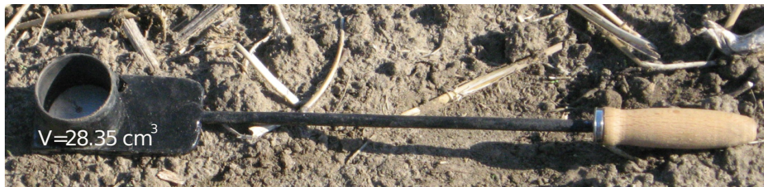
Fig. 6. Kit for measuring soil bulk density
