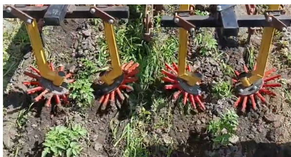
Figure 2. Operation of polyurethane finger-star discs in tomato rows.
