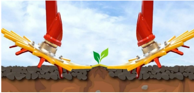
Figure 8. Technological scheme of operation of polyurethane rotary finger-star discs.
