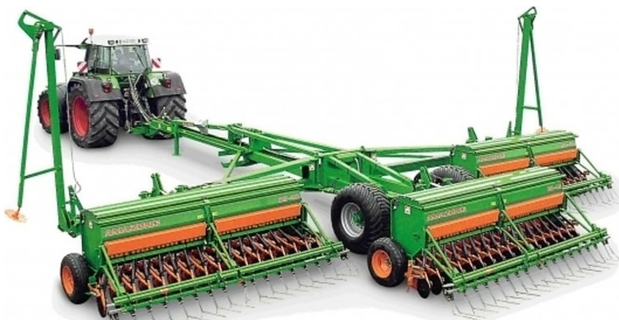
Fig. 1 Three-machine (three-module) trailed sowing machine-tractor unit
