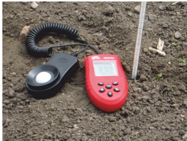
Fig.4. Instruments for measuring illumination and soil temperature
