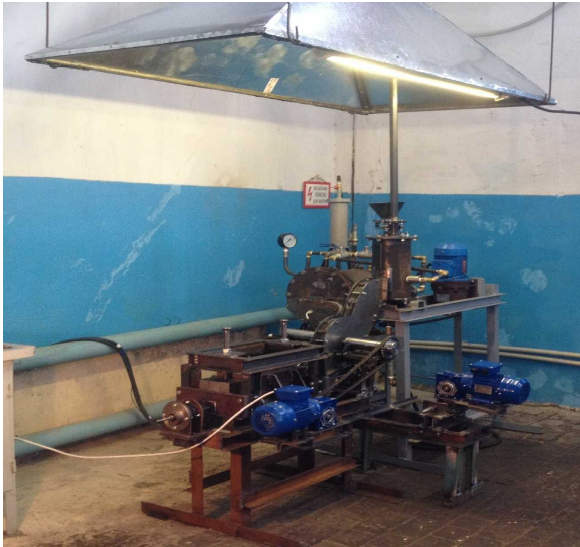
Figure 2. Overall view of the experimental complex for oil extraction from oil-bearing raw material
