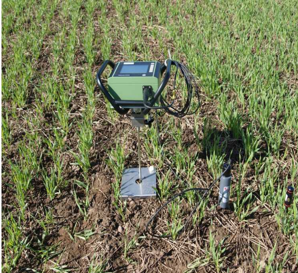
Fig. 4. Eijkelkamp Penetrologger for measuring of cone or penetration resistance (up to 70 cm), and at the same time is available to measure volumetric water or moisture content (up to 10 cm) [22].
