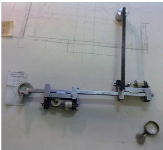
Fig.2. Determining the area of the blot ( \text{mm}^2 ) by planimeter
