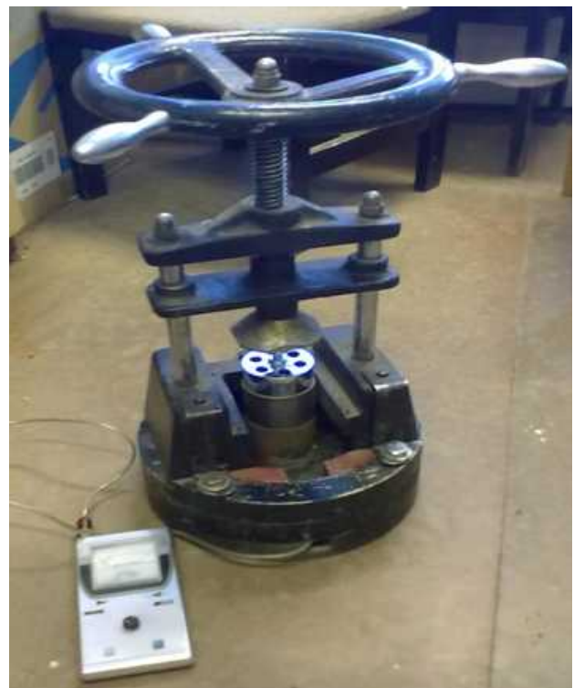
Fig.3. Oedometer for determining of the strain (kPa) in soil. The strain is measured by apparatus through strain-gage sensor (author E.P. Kuznetsova, AFI, compiled by Rein Põldoja, ECRI).
