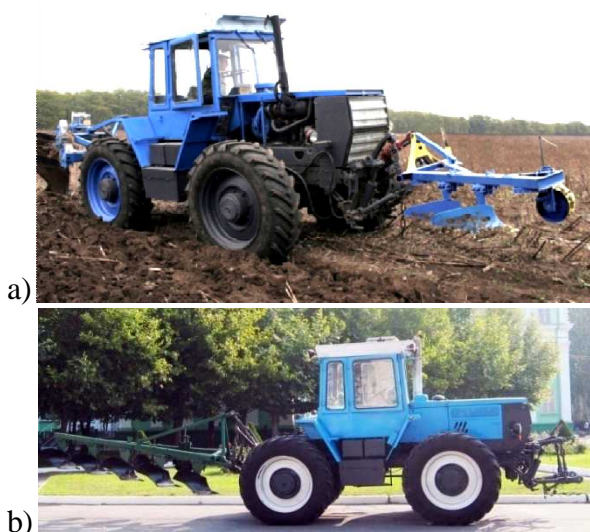
Figure 1. '2 + 4' (a) and '0 + 5' (b) ploughing combinations
