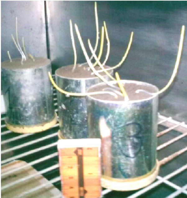
Fig. 1. Example of gutta liquids on the sprouts: in cylinder No 1 – soil is over compacted (not yet liquid); in cylinder No 2 - sparingly compacted; in cylinder No 3 – not compacted (actually the soil is loosening).
