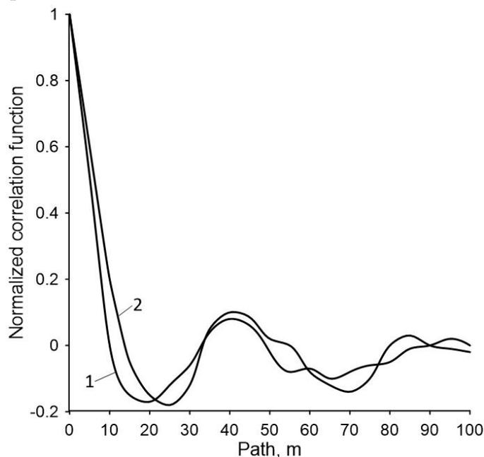
Fig. 4. Normalized correlation functions of fluctuations in the width of the sunflower row protective zone when MTU moves at different speeds: 1 –  $1.9 \text{ m}\cdot\text{s}^{-1}$ ; 2 –  $2.4 \text{ m}\cdot\text{s}^{-1}$
