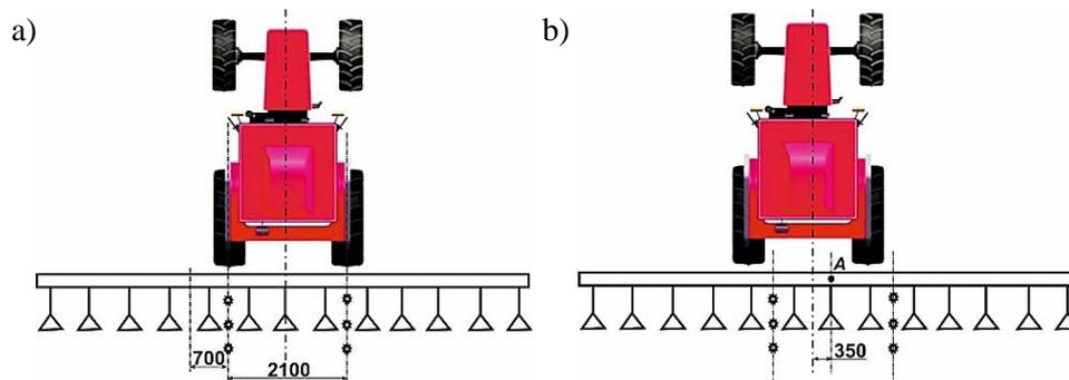
Fig. 1. Symmetric (a) and asymmetric (b) diagram joining of the HTZ-16131 tractor with a 12-row row cultivator
