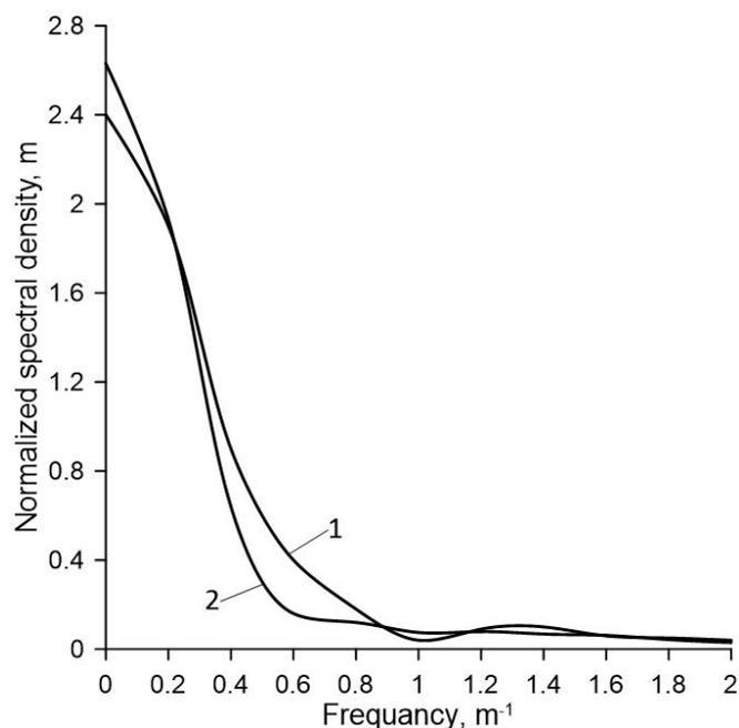
Fig. 5. Normalized spectral densities of fluctuations in the width of the sunflower row protective zone when MTU moves at different speeds: 1 –  $1.9 \text{ m}\cdot\text{s}^{-1}$ ; 2 –  $2.4 \text{ m}\cdot\text{s}^{-1}$
