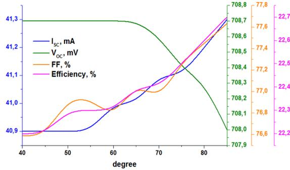
**Fig. 4.** Dependence of optoelectric parameters of the ZnO/porous-Si/Si heterostructure on the angle of texturing of the photovoltaic converter surface
