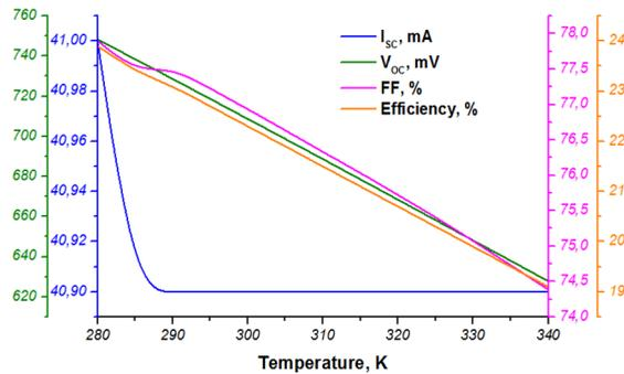
**Fig. 5.** Optoelectrical parameters of the photovoltaic converter based on ZnO/porous-Si/Si heterostructure at different temperature values
