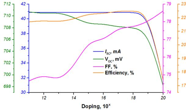
**Fig. 3.** Dependence of optoelectrical parameters of ZnO/porous-Si/Si heterostructure on the level of doping of ZnO coating
