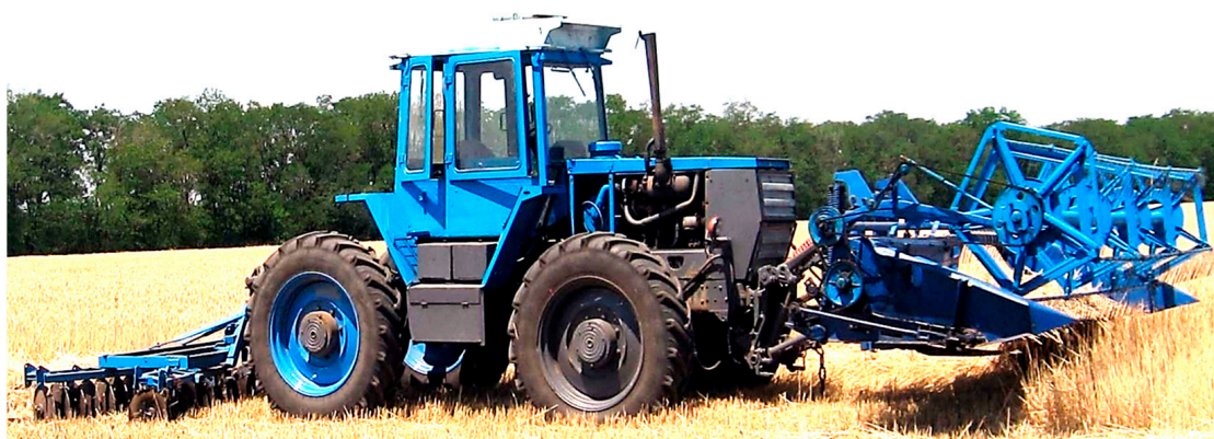
Figure 2. Harvesting unit with tractor's front-steering wheels.
