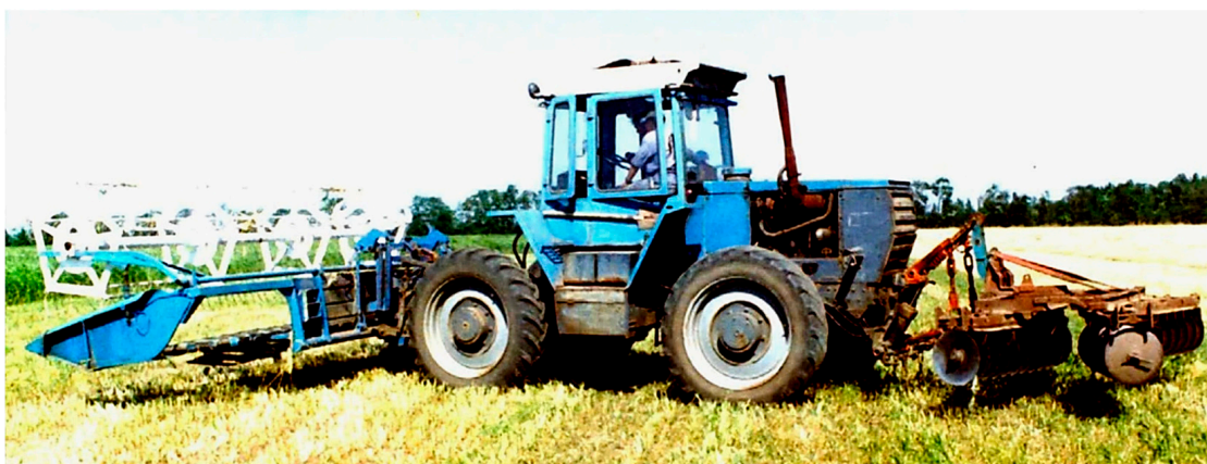
Figure 3. Harvesting unit with tractor's rear-steering wheels.
