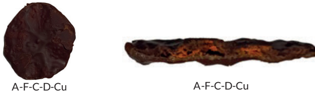
Fig. 5.6 The appearance of the A-F-C-D-Cu sample from the base layer side and its cross-section
