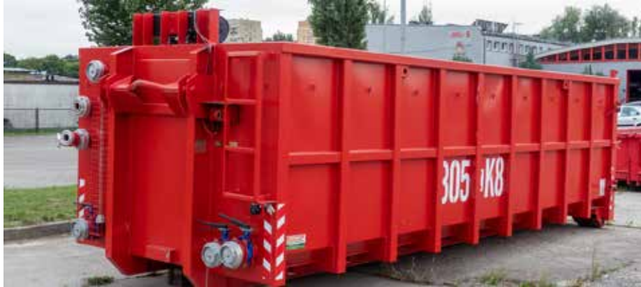
Fig. 1. Container for extinguishing electric vehicles [1]
