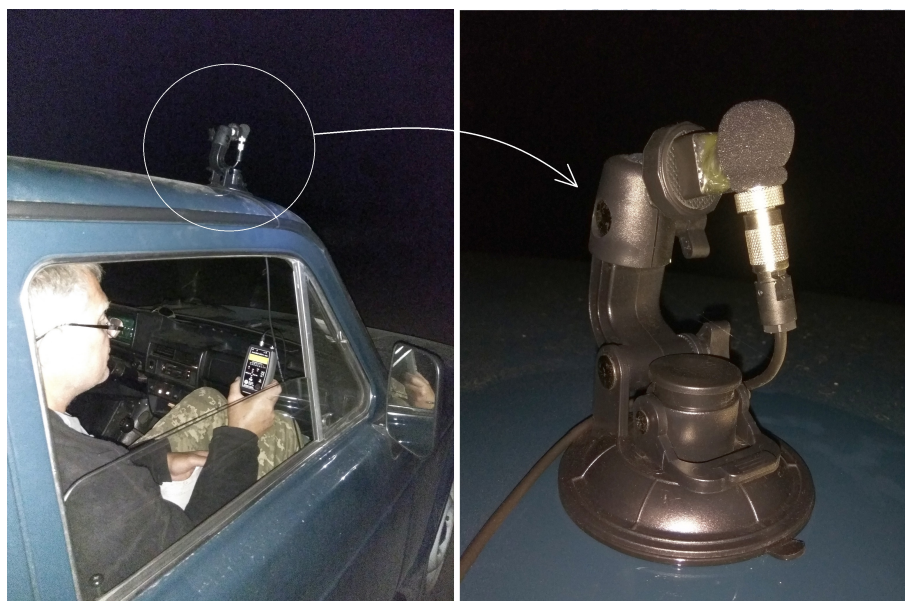
Figure 2. Using the LunaBat DFR-1 Pro detector with an external microphone on the Zaporizhia wind park transects in 2019.
