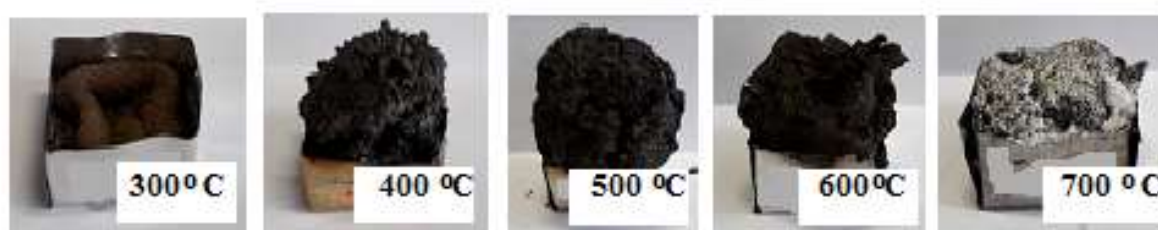
Figure 2. Samples of IK 6 intumescent coating after thermal treatment in muffle furnace
