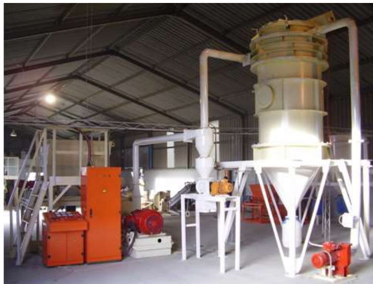
Figure 4. Installation of fine grinding of vegetable waste.
