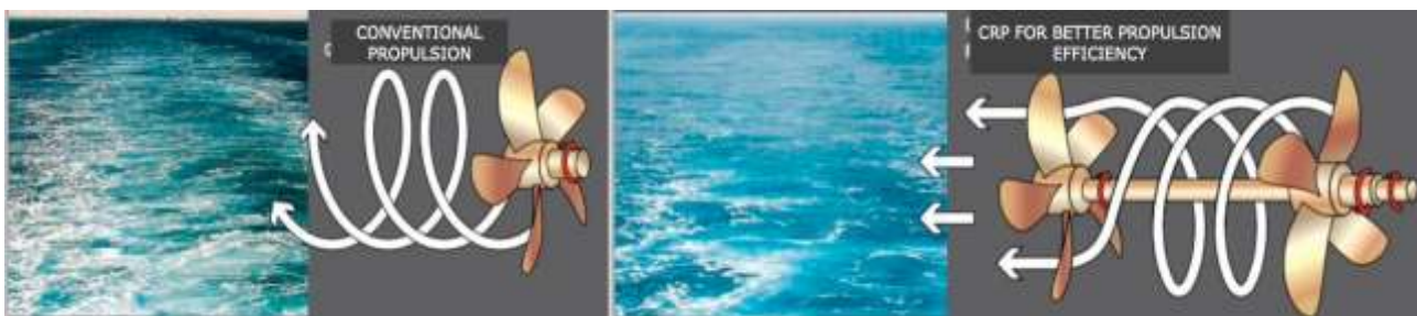
Figure 3. Conventional and contra-rotating propeller
