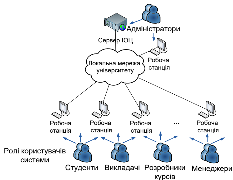
Figure 4. The system MOODLE scheme of work
