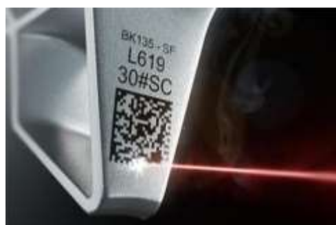
Figure 3. Direct laser marking technology
