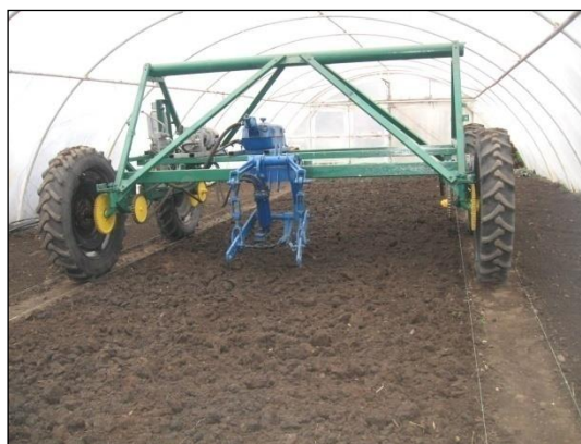
Figure 1 Bridge-type agricultural equipment with pneumatic wheels moving along the soil tracks of a permanent tramline
