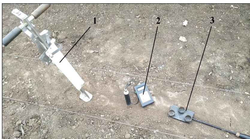
Figure 2 Measuring instruments for determining the physical and mechanical properties of the soil in traces of a permanent tramline: 1 – hardness tester of the Revyakin system; 2 – hygrometer MG-44; 3 – densitometer
