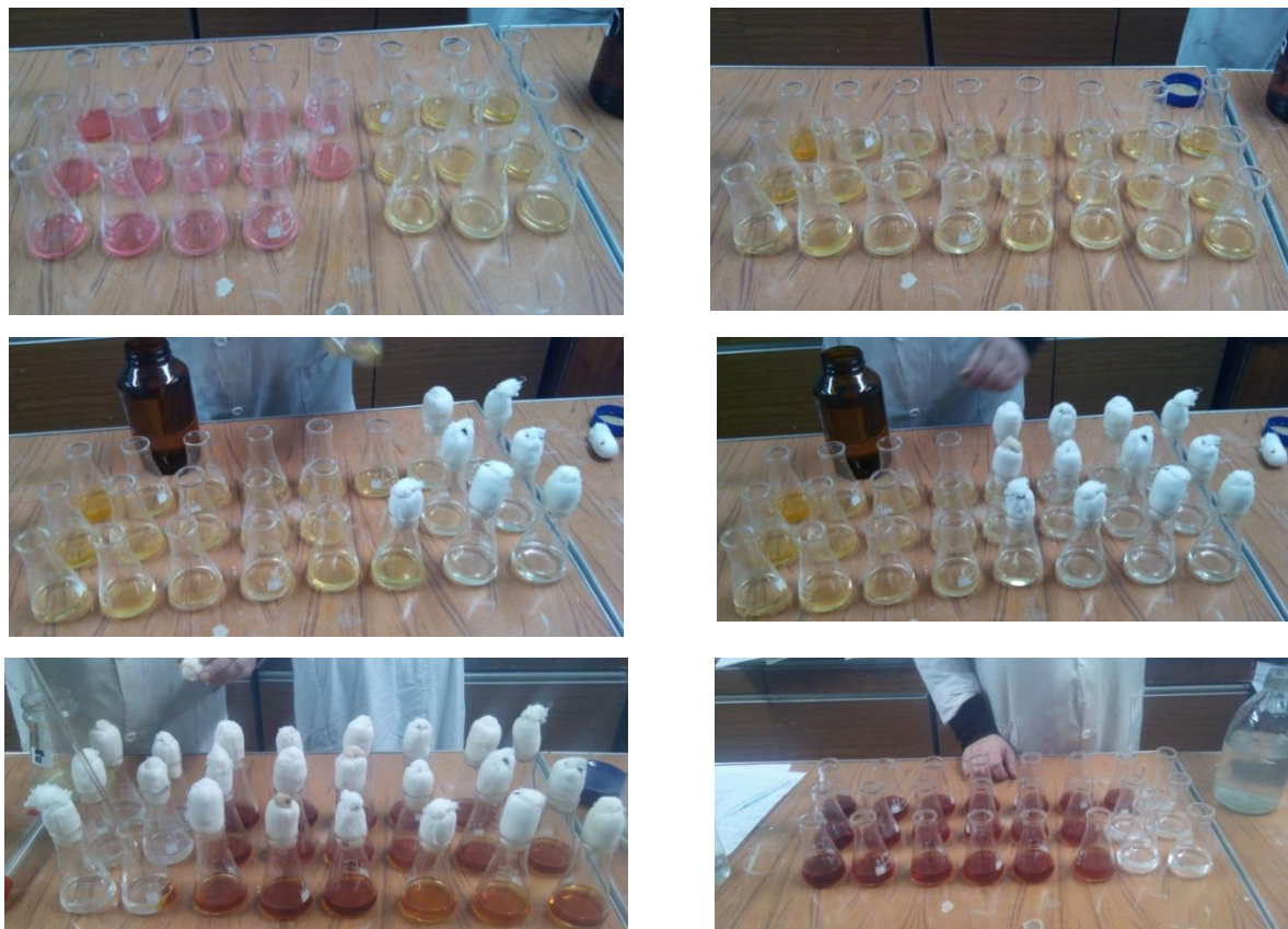
Fig. 3 – The process of determining the total nitrogen content by titration
